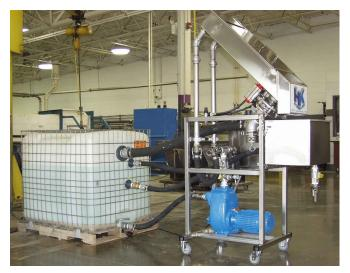
The high-capacity **HYDRAKLEEN** relies primarily on gravity for separation. It's a fully-packaged system in all stainless steel or polypropylene construction on an adjustable-height mobile stand, complete with filtration elements, optional pump and
