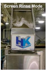
In **normal run mode**, the **HYDRAKLEEN** pumps the solid-containing liquid from a tank or process line, releasing it at the top of a hillside shearing screen. In flowing down the screen, the liquid is filtered by shearing it to the underside of the screen while the solids propel automatically down the screen face under gravity to a collection basket. The filtered liquid flows back to the process tank through a main gravity return line.
